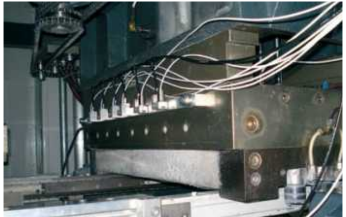
Small optris CT LT sensing heads installed in a machinery with a laminar air purge collar.
