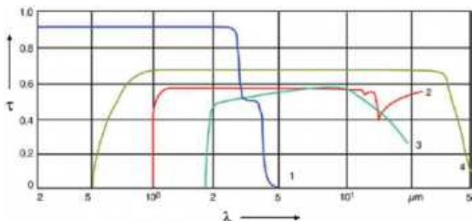
Transmissivity of typical infrared materials (1 mm thick)
