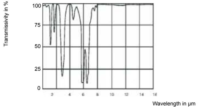
Spectral transmissivity of air (1 m, 32°C, 75 % r. F.)
