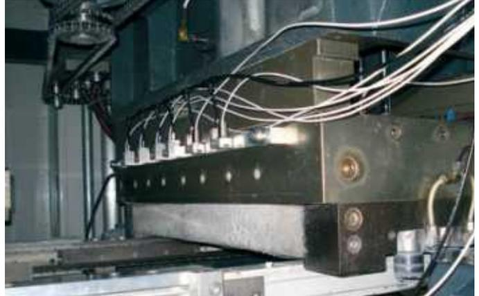
*Small optris CT LT sensing heads installed in a machinery with a laminar air purge collar.*
