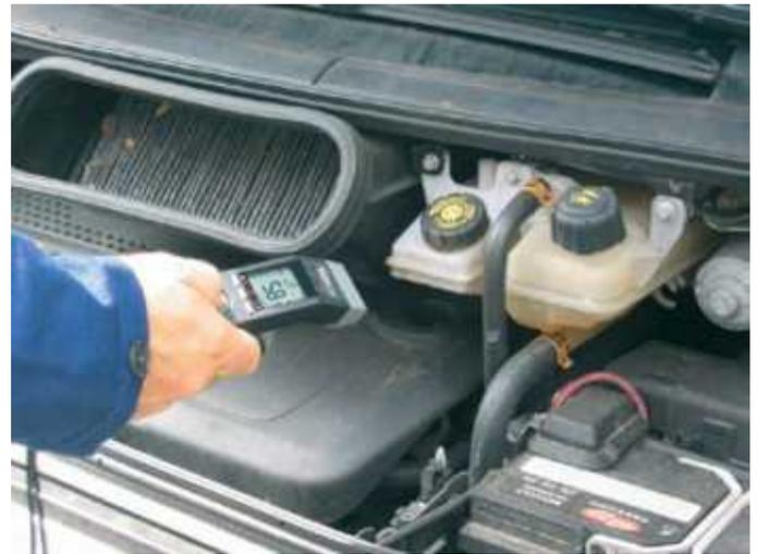
*Checking the heating system*
