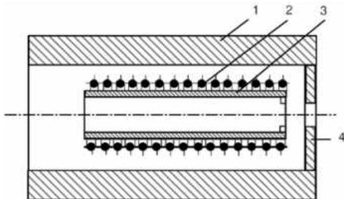
Drawing of a black body: 1 - ceramic conduit, 2 - heating, 3 - conduit made from Al<sub>2</sub>O<sub>3</sub>, 4 - aperture
