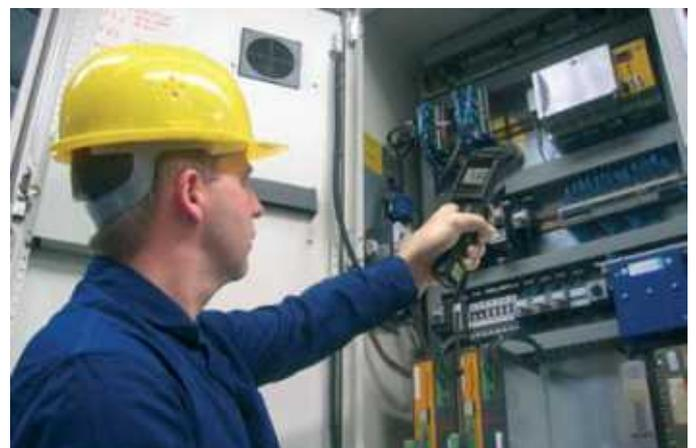
Detailed infrared temperature measurement of an electric control with the help of the installed close focus optics for 1 mm ranges of the optris LS LT
