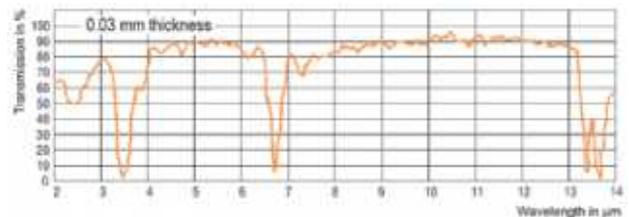
Spectral permeability of plastics made from poethylene.
