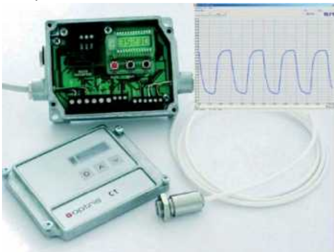
The output interfaces of infrared thermometers may be directly connected with PC, laptop, measuring data printer. PC software allows customer oriented graphics and tables.
