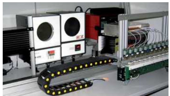
Automated calibration stations at Optris GmbH
