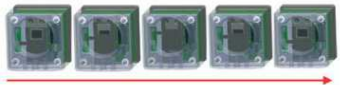
For offset compensation the whole field of view of an infrared sensor array is closed by a linear motor for a short time
