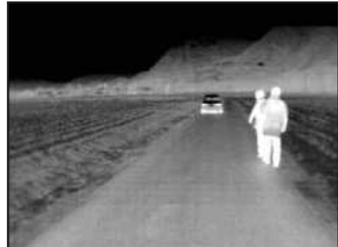
Figure 15: Infrared cameras are now available as an option on many new cars for improved night vision.
