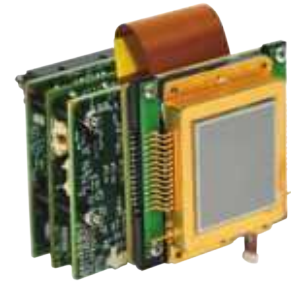
Figure 7: A high resolution 1024x768 uncooled core for high performance military and commercial infrared imaging applications.
