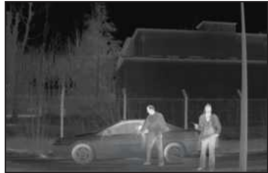
Figure 1: Thermal image obtained with 1024x768 a-Si microbolometer detector shows both high sensitivity and resolution. Courtesy ULIS.
