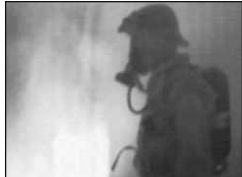
Figure 11: Because infrared cameras can see through smoke, they are a valuable tool for firefighters.
